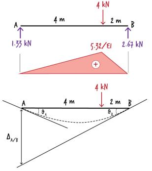
Figure 9: Vertical distance between two tangent lines at the left end of a beam
