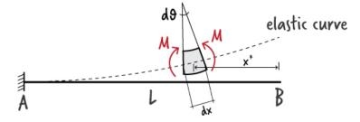
Figure 10: An infinitesimal beam element at an arbitrary position in a beam
