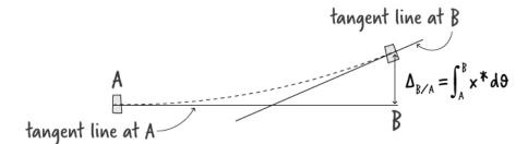
Figure 12: The vertical distance between the tangent lines at two distinct points in a beam
