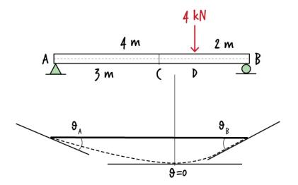
Figure 7: The elastic curve for a beam subjected to an asymmetrical loading
