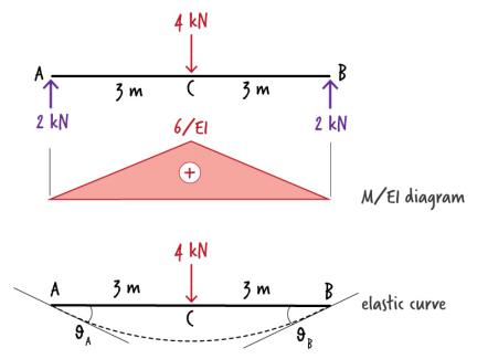
Figure 6: The M/EI and elastic curve diagrams for a simply supported beam
