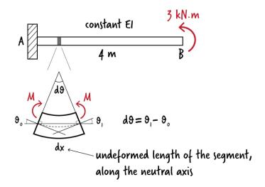
Figure 3: An infinitesimal deformed beam element
