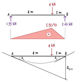
Figure 8: Vertical distance between two tangent lines at the right end of a beam
