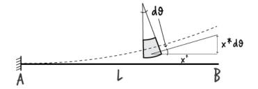
Figure 11: The vertical distance between the end tangent lines of a beam element
