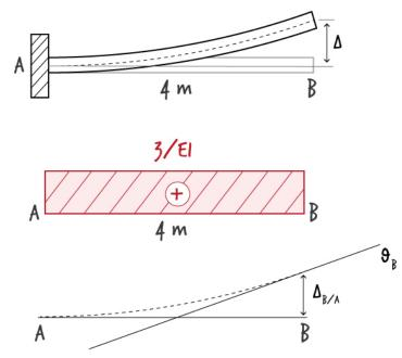
Figure 13: The M/EI diagram and the elastic curve for a cantilever beam
