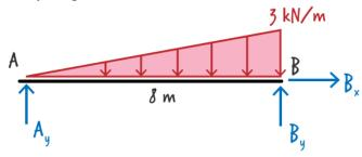
Replace the distributed load with its equivalent concentrated load. The magnitude of the concentrated load is equal to the area of the triangle; the location of the load is the geometric center of the triangle.
