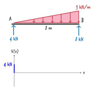
Shear at the right end of the beam equals shear at the left end minus the area of the triangle representing the load. The area is (3 kN/m)(8 m)/2 = 12 kN. So, shear at the right end of AB equals 4 - 12 = -8 kN.
