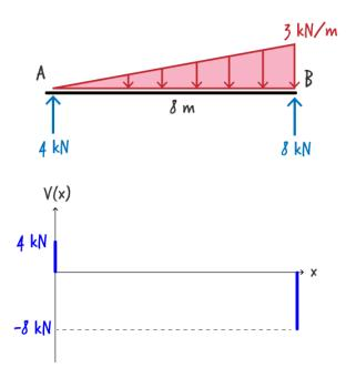
Since the load varies linearly, the shear diagram is going to have a linearly varying slope. This means, the diagram itself takes the shape of a quadratic equation (a second-degree polynomial) which has a linearly varying slope.
