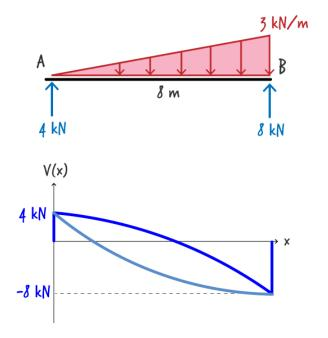
Note that the quadratic curve can be drawn in two ways. In the above diagram, the curve shown in light blue has an increasing slope. At A the curve has a large negative slope which increases toward zero as we approach Point B. The curve shown in dark blue has a decreasing slope. Its slope is close to zero at A, and becomes more negative as we approach B.
