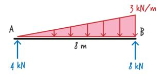
To draw the shear diagram, we start from the left end of the beam. Shear at the left end of AB is positive 4 kN, since there is an upward force of 4 kN at A.
