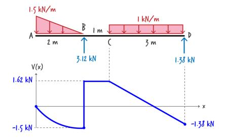
Finally, since there is an upward concentrated force of 1.38 kN at D, shear jumps from negative 1.38 kN to zero at that point.
