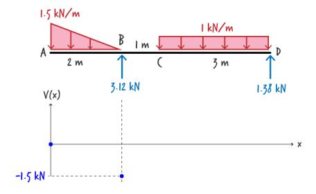
Since the load varies linearly in segment AB, the shear diagram is going to have a linearly varying slope in that segment. This means, the diagram itself takes the shape of a quadratic equation (a second-degree polynomial), which has a linearly varying slope.
