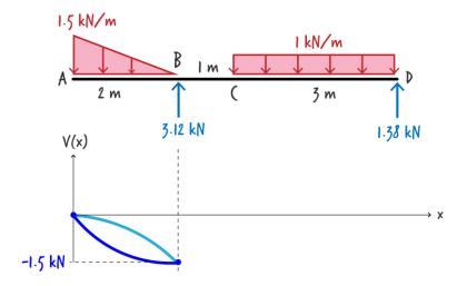
To determine which curve correctly represents the shear diagram, we need to examine the free-body diagram. If the distributed load is increasing in value as we move from A to B, then the curve with an increasing slope is the correct shape. However, if the load is decreasing in value from A to B, then the correct curve has to have a decreasing slope.
