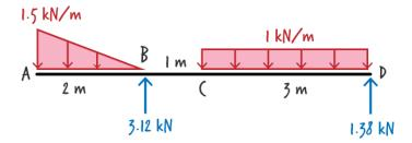
To draw the shear diagram, we start from the left end of the beam. Shear at the left end of AB is zero, since there is an upward concentrated force at A.
