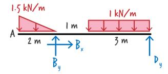
Replace the distributed load with its equivalent concentrated load. The magnitude of the concentrated load equals the area of the triangle representing the load, and the location of the load is the geometric center of the triangle.
