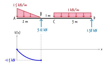
At B, there is going to be a jump of 3.12 kN in shear value due to the upward force present at that point. This means shear at the right side of B is 1.62 kN. Shear remains constant throughout BC since the segment is not subjected to any loads.
