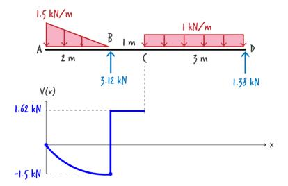
As the above diagram indicates, shear at the left side of Point C equals 1.62 kN. And since there is no concentrated force present at C, shear to the right of the point is also 1.62 kN.
