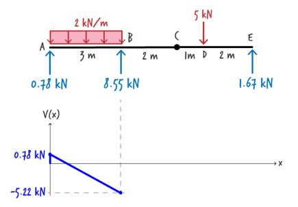
The upward concentrated force at B causes a jump in the shear value. The amount of increase is equal to the magnitude of the upward force; it is 8.55 kN. So, shear jumps from negative 5.22 kN to positive 3.33 kN.
