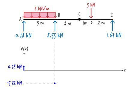
Since the distributed load acting on AB is constant, the shear diagram is going to be a straight line in the segment, as shown below.
