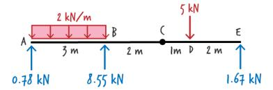
To draw the shear diagram, we start from the left end of the beam. Shear at the left end of AB goes from zero to 0.78 kN, since there is an upward concentrated force with that magnitude at A.
