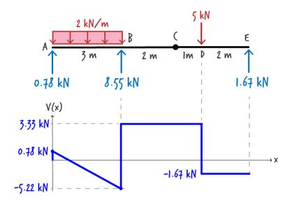
Finally, shear returns to zero at E, since there is an upward reaction force of 1.67 kN at the right end of the beam.
