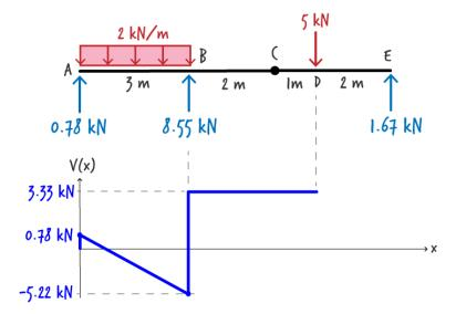
The downward force of 5 kN at D causes a drop in shear value by that amount. So, shear drops from positive 3.33 kN to negative 1.67 kN at D. Then, since DE is not subjected to any external loads, shear remains constant throughout that segment.
