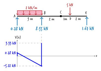
Then, since no load is acting on segments BC and CD, shear remains constant throughout that length of the beam.
