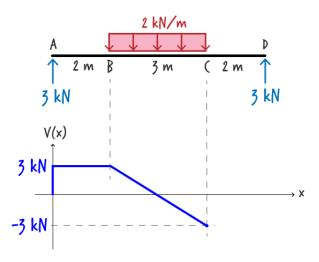
Shear remains constant in segment CD since there is no load acting on the beam from C to D.
