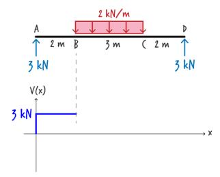
For segment BC, shear at the left end of the segment is 3 kN. To determine shear at the right end of the segment, we subtract the area under the load diagram from 3 kN. The load area is that of the rectangle representing the load, it equals (2 kN/m)(3m) = 6 kN. So, shear at the right end of AB equals 3 - 6 = -3 kN. Since the load is uniformly distributed over the segment, shear is going to be represented using a straight line.
