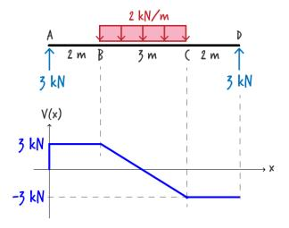
Then, shear goes back to zero since there is an upward force of 3 kN at the right of the beam.
