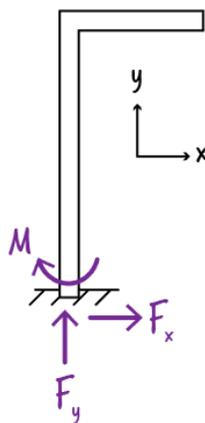
Figure 6: Reaction forces associated with a cantilever frame
