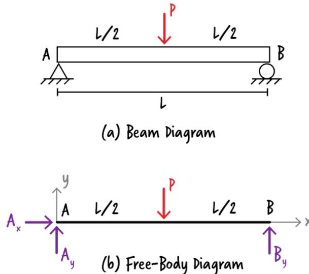
Figure 7: A simply supported beam and its free-body diagram
