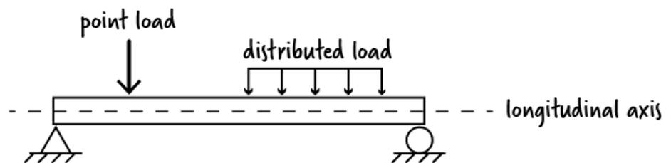
Figure 1: A beam subjected to a point load and a uniformly distributed load
