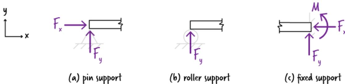
Figure 4: Reaction forces associated with each support type
