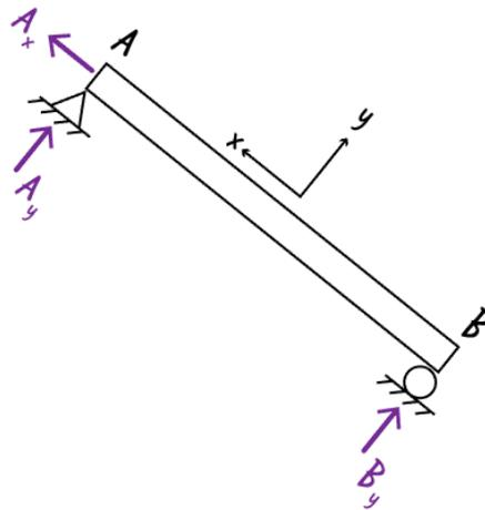
Figure 5: Reaction forces associated with a simply supported beam
