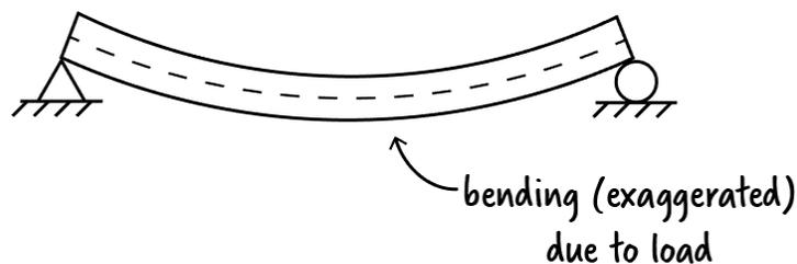
Figure 2: Bending of a beam due to applied load(s)
