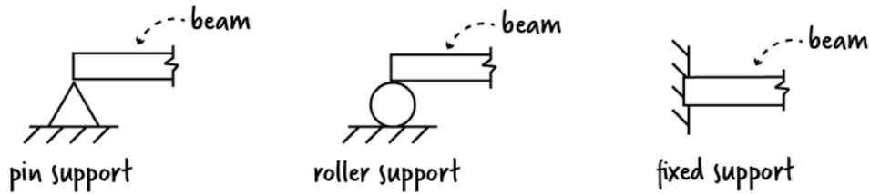
Figure 3. Common support types in beams
