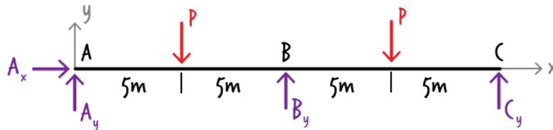
Figure 11: The free-body diagram for a beam with three supports
