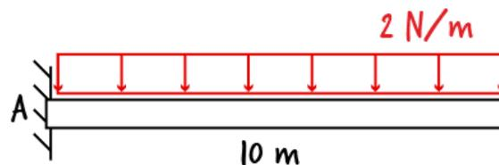
Figure 8: A cantilever beam subjected to a uniformly distributed load
