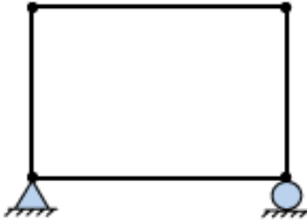
Figure 9: A rectangular truss with four members
