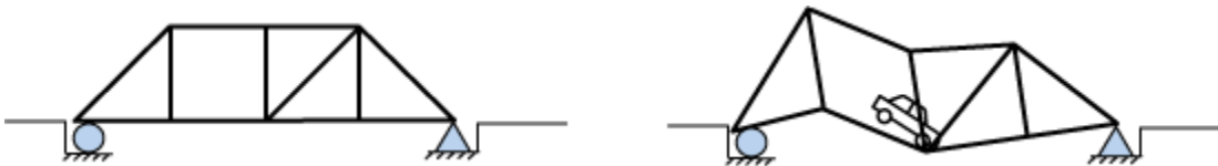
Figure 2: An unstable truss and its collapsed configuration
