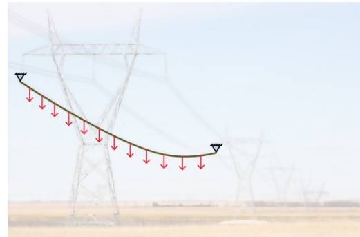
Figure 4: A power line and its line drawing characterization as a cable hanging freely under its own weight
