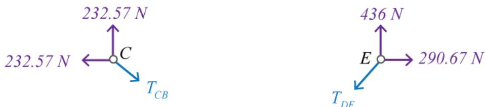
Figure 28: Free-body diagrams of two support points in a cable system
