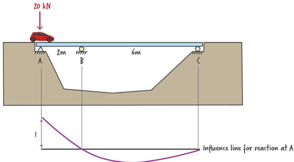
Figure 12: Load position for creating the maximum upward reaction at A
