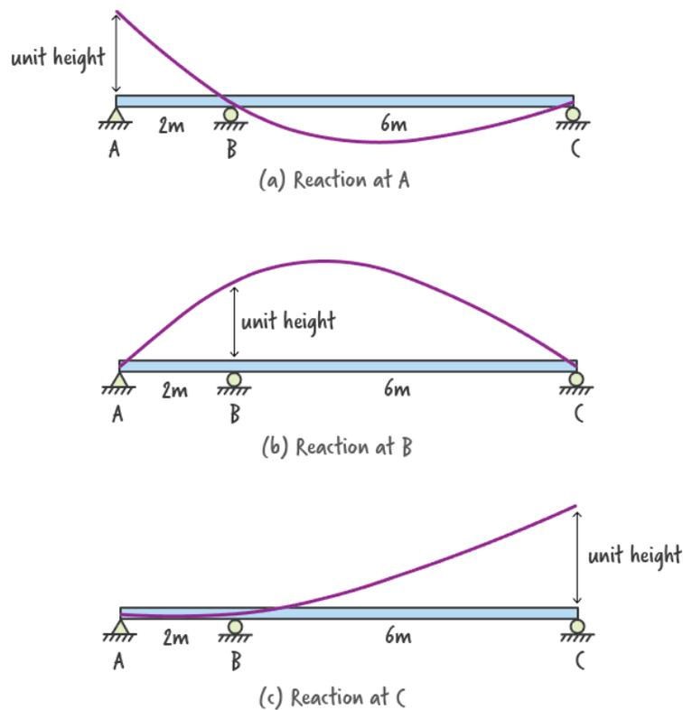
Figure 1: Reaction influence lines for the beam
