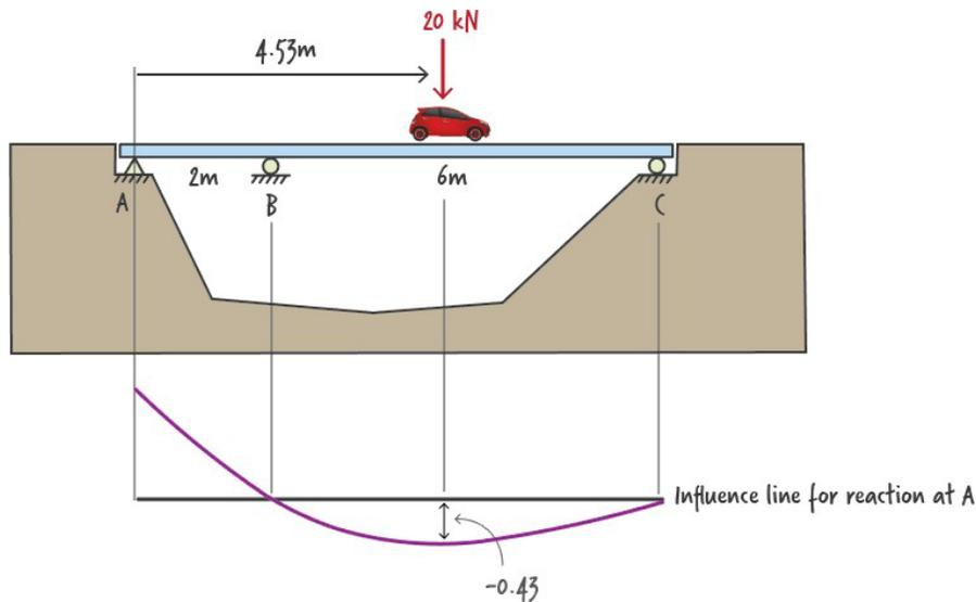
Figure 13: Load position for creating the maximum downward reaction at A
