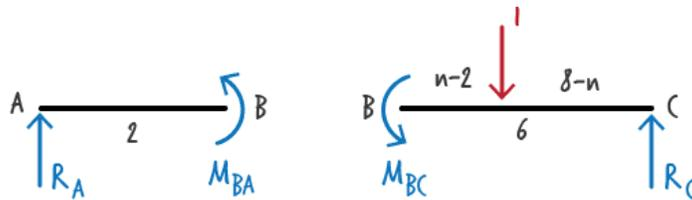
Figure 11: Free-body diagram of the beam segments for Equation Set 2
