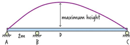
Figure 2: Location of the maximum height of the influence line for the reaction force at B
