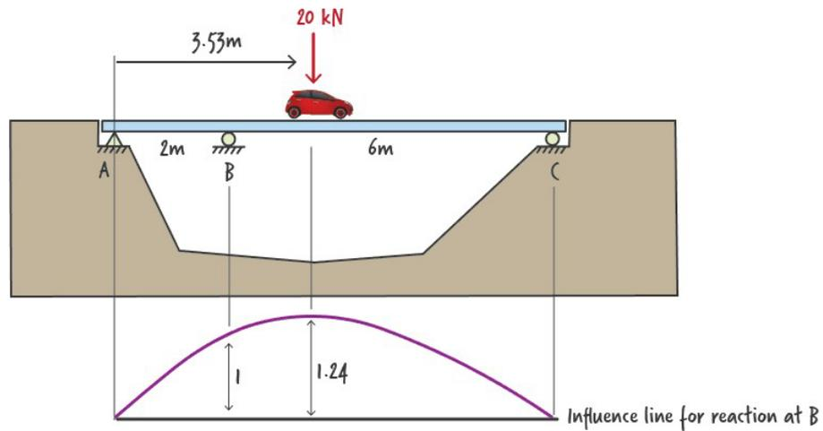
Figure 14: Load position for creating the maximum upward reaction at B
