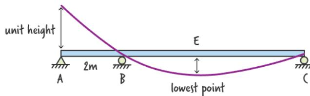
Figure 3: Location of the minimum height of the influence for the reaction force at A
