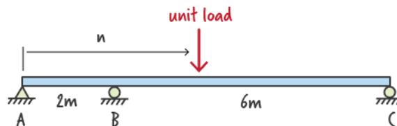
Figure 4: A two-span continuous beam subjected to a unit load
