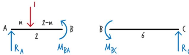
Figure 10: Free-body diagram of the beam segments for Equation Set 1
